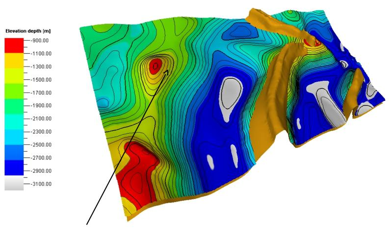
Injection point at ca. 1500 m depth at the flank of the anticline
