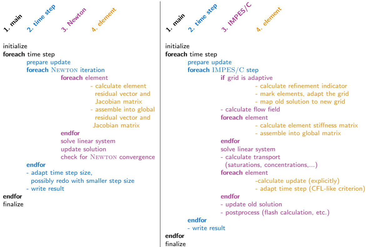
Figure 5.4: Structure of a fully implicit ( left ) and a sequential ( right ) scheme in DuMu x .
